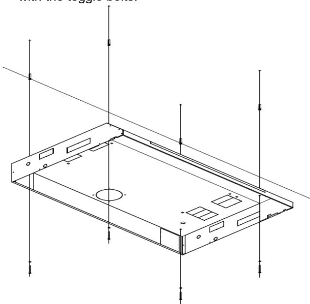
Then install the supporting brackets and the built-in version of the device (securing it through the 6 "B" holes, using the screws and washers supplied with the toggle bolts), install one of the TELESCOPIC AIR OUTLET DUCT kits DB0160/DB0164 and an EXTERIOR PANEL KIT FOR BUILT-IN CEILING INSTALLATION LC0618/LC0622, in accordance with the specific instructions contained in the kit itself.
