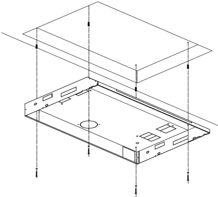
Then install the supporting brackets and the built-in version of the device (securing it through the 6 "B" holes, using the screws and washers supplied with the toggle bolts) and an EXTERIOR PANEL KIT FOR BUILT-IN INSTALLATION LC0578/LC0582, in accordance with the specific instructions contained in the kit itself.
