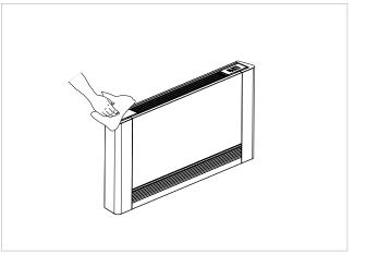
Clean the external surfaces using a soft cloth dampened with water.
