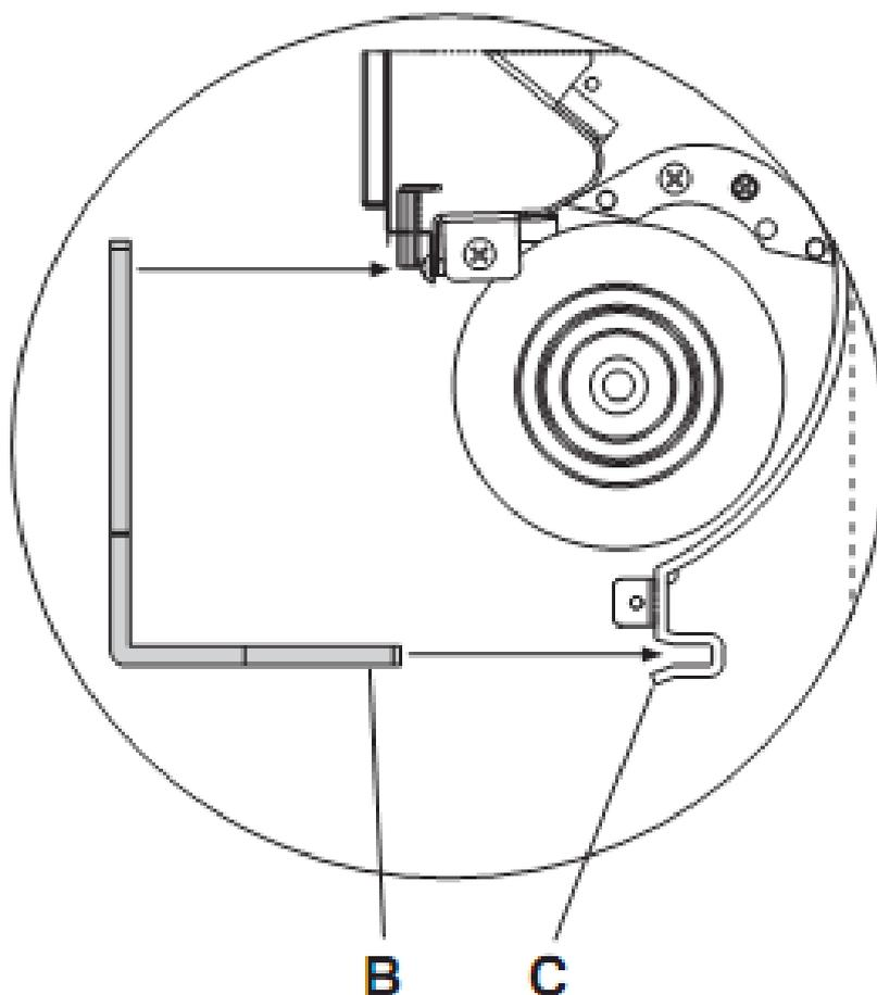
**!** Re-install the FILTER-STOPPER crossbar, securing it with the 2 screws previously removed in order to guarantee the safety of the device.
