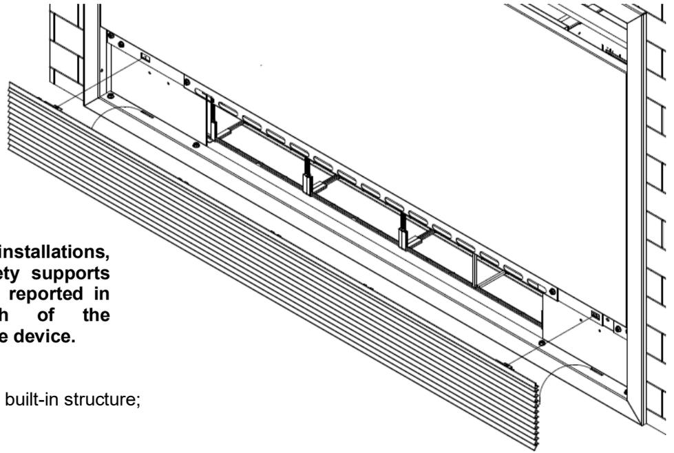
**!** For horizontal ceiling installations, install the front grill safety supports following the instructions reported in the relevant paragraph of the handbook supplied with the device.
