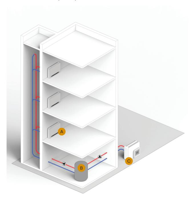
The air-source heat pump draws energy from the outside air to balance the loop. The temperature of the loop is at a temperature condition that allows very high seasonal efficiency to the air-to-water heat pump.
