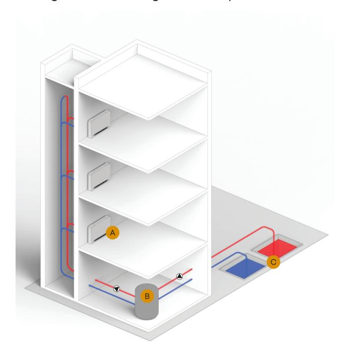
Groundwater, and even better geothermal probes, are very favorable temperature thermal sources that remain constant throughout the year. They allow thermal balancing of the plant loop in both winter and summer phases using 100% renewable energy.
