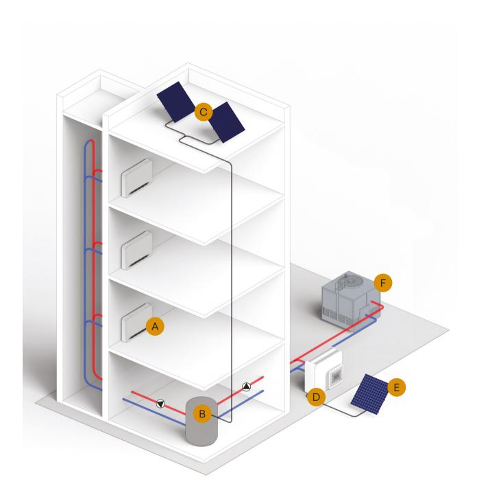
Solar thermal panels for heating the ring water in winter phase, evaporative tower for cooling the ring water in summer phase, photovoltaic panels to support the heat pump.
