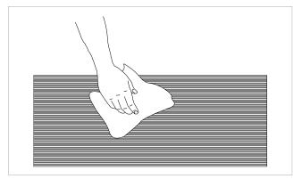
Clean the external surface of the grid using a soft cloth dampened with water.
